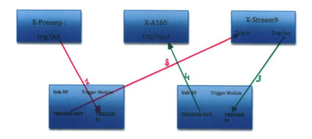
A trigger module : trigger converter bidirectional : 3,3V (SmartLine / X-Stream9) to 12V (X-Preamp / XA160/X-A220/X-CD1000/ XA1200)
