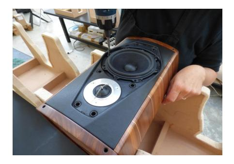
Unscrew the 8 screws that fasten the midwoofer to the cabinet using a T15 screwdriver.
