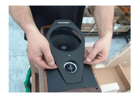
Carefully lift the front baffle up by covering its outline as shown in the picture.
