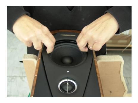
Carefully lift the front baffle up using your fingers as shown in the picture.
