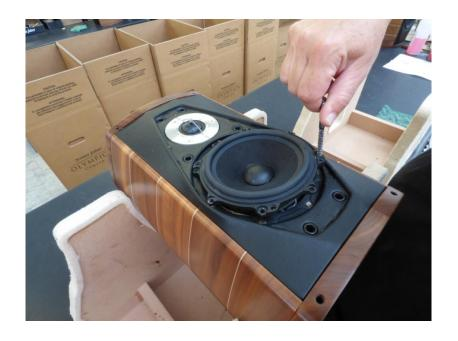
Lift the driver up using a big screw or a flatblade screwdriver. Pay attention not to ruin the leather coating.
