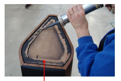
Do not spread this lower part with the glue. Spread the top surface with the supplied polyurethane (or silicon) glue the very way you see in this pic. Put the new glue on top of the old one.
